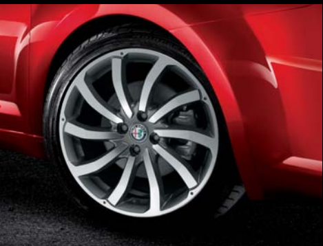
74A - 17" 10-spoke 'Turbine' design alloy wheels with 215/45 R17 tyres
