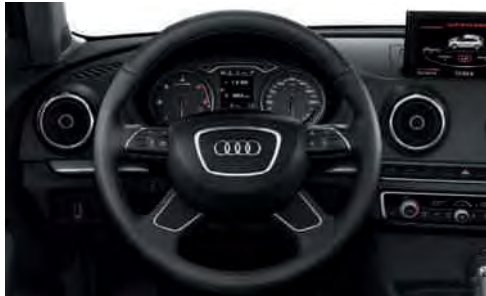
Multifunction leather steering wheel in 4-spoke design for operating the available infotainment features; adjustable in height and reach, with full-size airbag; with optional shift paddles for changing gears manually with automatic transmission
