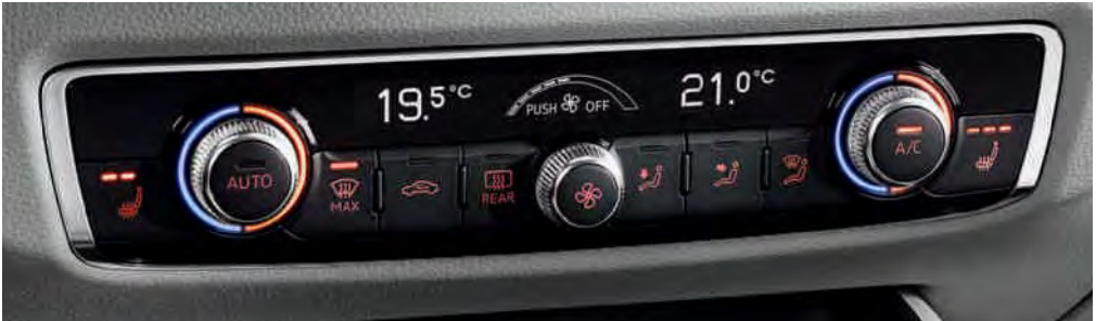
Deluxe automatic air conditioning electronically regulates the air temperature, flow rate and distribution; separate temperature control for driver and front passenger with indirect ventilation through defroster nozzles and sunlight-dependent control; automatic recirculation mode by means of air quality sensor, combined filter and rear vents; with humidity sensor and key-coded settings
