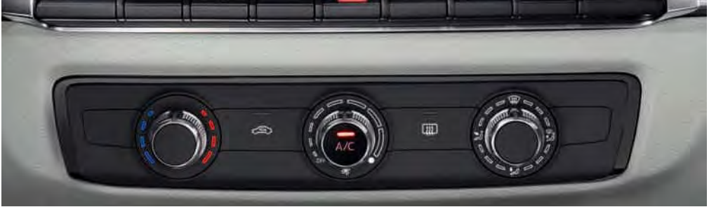
Air conditioning, manual cools or heats up the vehicle passenger compartment; manually adjustable air distribution, manual recirculation mode, infinitely variable blower and particulate filter; 4 round vents in the dashboard that can be individually adjusted to provide directed or diffuse air flow, footwell vents at the front and rear and defroster nozzles for the windscreen and side windows
