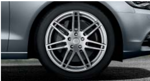
Audi exclusive cast aluminium wheels in 7-twin-spoke design size 8.5 J x 19 with 255/40 R 19 tyres. From quattro GmbH
