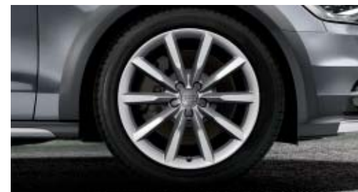
Cast aluminium wheels in 10-spoke design size 8.5 J x 19 with 255/45 R 19 tyres
