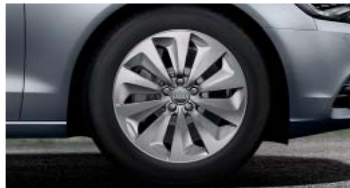
Cast aluminium wheels in 10-arm turbine design (hybrid design) size 8 J x 17 with 225/55 R 17 tyres
