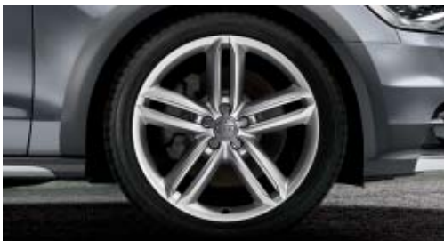
Cast aluminium wheels in 5-parallel-spoke design size 8.5 J x 20 with 255/40 R 20 tyres
