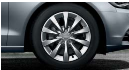
Cast aluminium wheels in 10-spoke design size 8 J x 17 with 225/55 R 17 tyres, optionally available with all-season tyres
