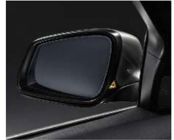
□ **Lane Change Warning System** detects vehicles in the driver's blind spot and vehicles approaching at speed in the adjacent lane when the driver has activated the indicator in order to change lanes. The system alerts the driver by making the steering wheel vibrate and by a visual warning on the exterior mirror.
