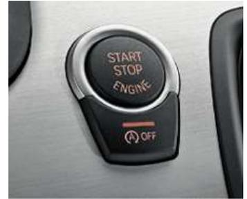
**Start/Stop button** for starting or stopping the engine after unlocking the car. The vehicle key is automatically recognised, without having to be inserted in the ignition (shown here: 520d with Auto Start/Stop function).
