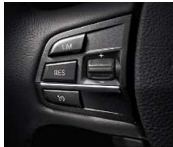
**Cruise Control with braking function** stores any desired speed upwards of approx. 30 km/h and maintains it. The speed limiting function warns the driver via a lamp in the instrument cluster and an acoustic signal when the selected speed is exceeded.
