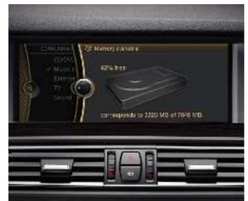
□ **Hard disk drive** enables quick access to a large collection of music files which can be transferred to the 12 GB hard disk from a CD, MP3 player or USB stick (included with Navigation system Professional\*).
