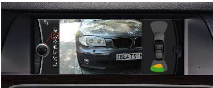
□ **Rear view camera** shows a clear image of the area behind the vehicle on the Control Display. Interactive tracking lines indicate for example whether or not the intended parking space offers enough room for the vehicle. The rear view camera is activated by engaging reverse gear.
