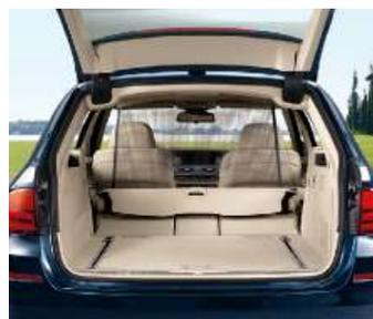
■ **Load area cover, complete with divider net:** when opening the tailgate or rear window, the comfort opening function lifts the load area cover up and out of the way, for convenient loading and unloading. The divider net prevents luggage from falling into the passenger compartment when braking heavily.
