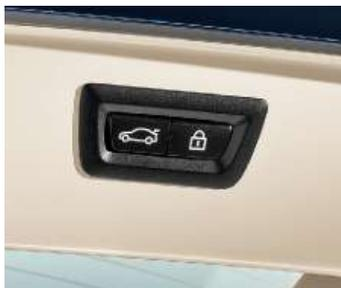
□ **Electric tailgate:** the tailgate can be opened automatically, using the remote control unit, and closed by pressing a button integrated in the edge of the tailgate. Opening is via an electrohydraulic mechanism. The load area cover is automatically raised when opening the tailgate, and lowered back into place when closing it.
