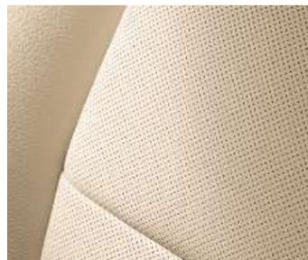
□ **Active seat ventilation** for driver and front passenger seats considerably enhances summer comfort by ensuring a pleasantly cool seat temperature. Ventilators in the seat surface and backrest blow air through the perforated leather seat covers.
