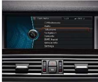
■ **Control Display** with high-resolution TFT colour monitor (7") for displaying functions that are accessed using the Controller. In conjunction with the optional Navigation system Professional\*, the screen measures 10.2" (shown here).
