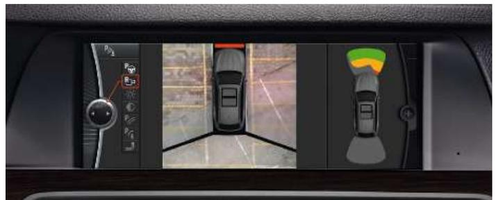
□ **Surround View** offers the driver a good view of the area directly around the vehicle when manoeuvring. The BMW is represented as seen from above on the Control Display. The rear view camera enhances visibility when reversing at speeds below 20 km/h, for example when parking (only in conjunction with rear view camera and PDC). The Side View function enhances visibility when joining a road from a side street or exit.
