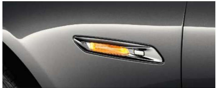
□ **Park Assistant** makes parallel parking easier. When travelling at speeds below 35 km/h, the system measures any parking gaps the vehicle passes. When a big enough gap has been found, the Park Assistant will do the steering, while the driver continues to operate the accelerator and brake pedals. The sensor is harmoniously integrated into the side indicator.
