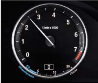
■ **BMW EfficientDynamics display.** As soon as the driver brakes or lifts the right foot off the accelerator, Brake Energy Regeneration converts the vehicle's redundant kinetic energy into electric energy and feeds this into the battery. This charging process is indicated by a symbol in the rev counter display.
