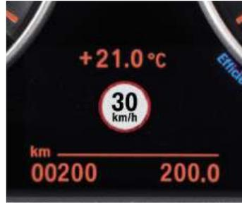
□ **Speed Limit Info** detects speed limits and shows the driver the currently applicable speed limit in the Info Display or the optional Head-up Display (only in conjunction with Navigation system Professional\*).
