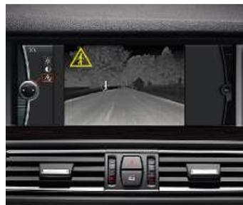
□ **BMW Night Vision with pedestrian recognition** uses an infrared camera to detect people and animals up to a distance of 300 metres. The camera images appear in the Control Display. The pedestrian recognition feature displays a visual warning (optionally shown in the Head-up Display) as soon as it detects people moving near the road. The infrared camera for BMW Night Vision is integrated in the kidney grille.
