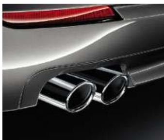
**Exhaust tailpipes:** the models 523i, 528i, 520d, 525d and 530d feature a visible twin tailpipe on the left; the 535i and 535d have two single tailpipes, one on the left and one on the right.
