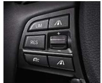
**Active Cruise Control with Stop&Go function** and approach warning incl. light-braking function. For enhanced comfort in stop-and-go traffic. Combines speed control with active distance control, slowing the car down to a stop if needed, and starting it up again in standard stop-and-go situations.
