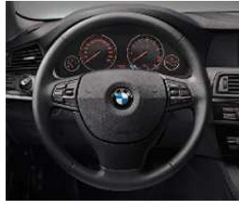
**Leather steering wheel** with multifunction buttons enables comfortable control of many different functions, without having to take one's hands off the wheel. The buttons on the left cover the complete set of cruise control functions; those on the right are for audio functions such as the radio and telephone.
