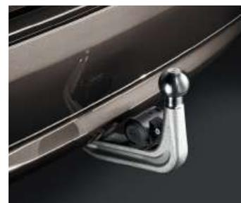
□ **Trailer tow hitch** with electrically adjustable ball head.
