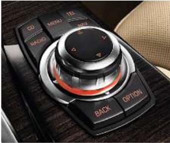
■ **Controller** is the central operating element of iDrive, and used to access all functions of the Control Display. Four frequently used menus can also be opened via the direct menu control buttons: CD, radio, navigation and telephone. In addition, eight functional bookmarks can be assigned functions of your choice.
