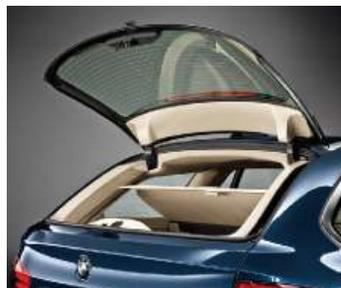
■ **Separately opening rear window:** for quick and easy access to the luggage compartment, the rear window can be opened separately, using the remote control unit. Handy: as the window lifts up, the load area cover is raised as well, and when manually closing the window, the load area cover is automatically lowered back into place.
