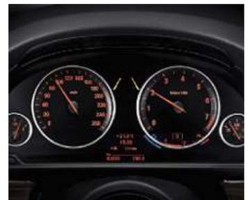
**Instrument cluster** with four analogue displays – speedometer, tachometer, fuel gauge and engine oil temperature – with a high-resolution Info Display in landscape format (5.7") below. This displays data such as current fuel consumption, on-board computer functions and, in combination with the Navigation system Professional\* or Business\*, navigation instructions.
