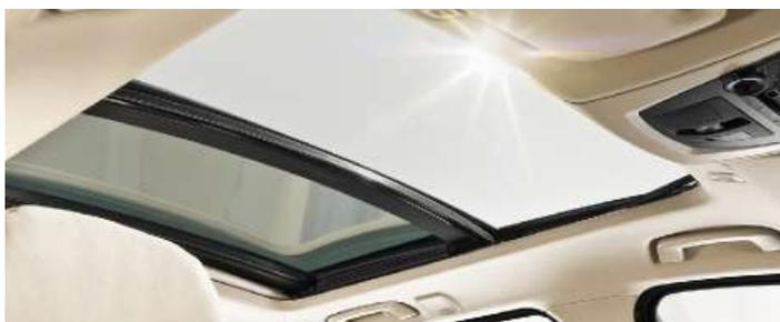
□ **Panorama glass roof** with generous aperture and viewing area and wind deflector. The front glass section can be raised electrically, using the vent function, and also comes with a sliding function, along with a floating headliner that provides protection from the sun, and a comfort opening/closing function with trap release.
