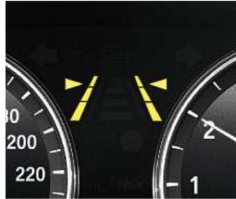
□ **Lane Departure Warning System** uses a camera to recognise whether the vehicle is threatening to stray outside the limits of the lane and alerts the driver by making the steering wheel vibrate.
