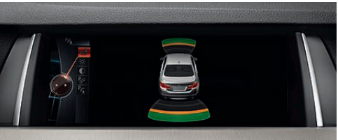
Rear-view Camera shows on the Control Display the area behind your vehicle. Guidelines indicate if your vehicle can fit in a parking space, and display parking turn angles. The Rear-view Camera is activated by engaging reverse gear. Park Distance Control (PDC) helps you judge distance to other vehicles and unseen objects when parking. The warning beeps come faster as the bumper approaches the object, turning into a constant tone at less than 12 inches. Side- and Top-view Cameras display video images of traffic approaching the front of the vehicle from the sides, such as when exiting a garage or parking space. The Top-view Camera provides birdseye video images of the road alongside the doors, taken by cameras positioned in the exterior mirrors.
