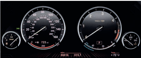
Black Panel Display shows a matte black surface when the ignition is off, with only the chrome rings of the circular instruments visible in 3-D. Switched on, the graphics display lights up, showing the trip computer and Check Control information; below the four analog dials is a high-res, wide-format Info Display that shows Navigation instructions, music tracks, etc. When ECO PRO mode is active, ECO PRO tips use graphics to encourage a more efficient driving style.
