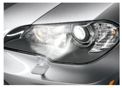
High-intensity, retractable headlight washers help keep lights clean of ice, mud, road salt and other coatings, for maximum road lighting and enhanced driving visibility.
