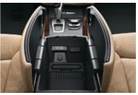
■ Auxiliary input port lets you connect an external audio source, such as an iPod<sup>®</sup> or MP3 player.
