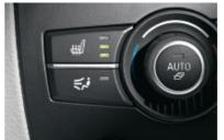
Heated front seats are a welcome feature in cooler weather. With the touch of a button, driver and front passenger can individually select from three heat settings.
