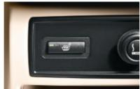
Heated rear seats are a welcome feature for left and right rear-seat occupants in cooler weather. With the touch of a button, passengers can individually select their preferred level of warmth. (Must be ordered with Cold Weather Package or optional heated front seats; not available with Leatherette upholstery.)
