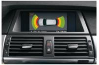
Park Distance Control, front and rear, makes parking and maneuvering in tight spaces easy. The sensors emit a beeping sound as they approach another vehicle or object. The signal increases in intensity the closer your bumper gets to the object.
