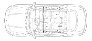
All dimensions in millimetres. The dimensions shown are mean values and apply to the standard-specification, unladen CLA 180.
