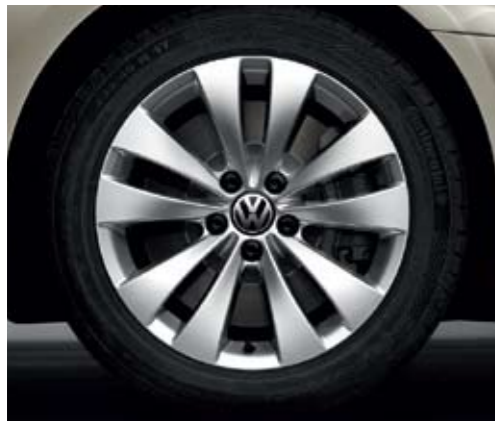
'Phoenix' 7½ x 17 with 235/45 R17 ContiSeal (self-sealing) tyres and anti-theft wheel bolts. Standard on Passat CC models and not available as an option.
